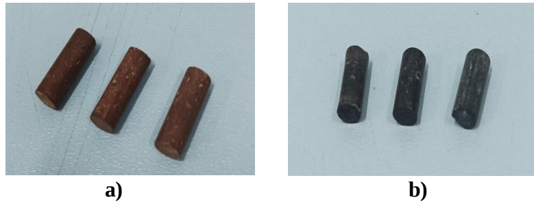
Figure 1. Specimens used in friction tests: a) bronze-reinforced composite and b) brass-reinforced composite
